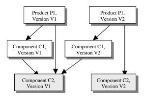
Figure 8. An inconsistent component integration.
