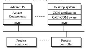
Figure 4. Many different components and products use the OMF component.
