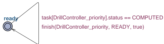
Fig. 27. Timed automata for DrillController actor functional behavior
