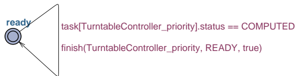
Fig. 24. Timed automata for TurntableController actor functional behavior
