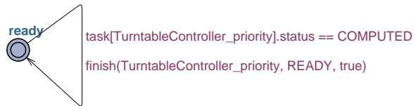
Fig. 26. Timed automata for TurntableController actor functional behavior
