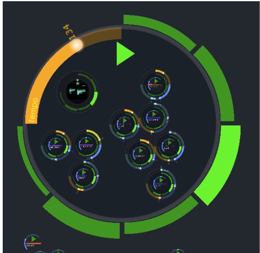
Figure 3. The performance item component. The green controllers around the component play different phrases. Similar controllers enable (or disable) media content in phrases. Media content can be surrounded with unit effects for image and sound processing. The line width of surrounding circle is proportional to the audio output, looking like a vibrating loudspeaker. Sliders run clockwise from lowest to highest value.
