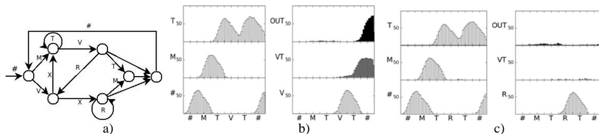
**Figure 1:** a) Finite State Machine (FSM) defining Reber grammar. Minicolumn model activity b) grammar string is recognized by the network c) a random string does not excite the OUT node above the recognition level
