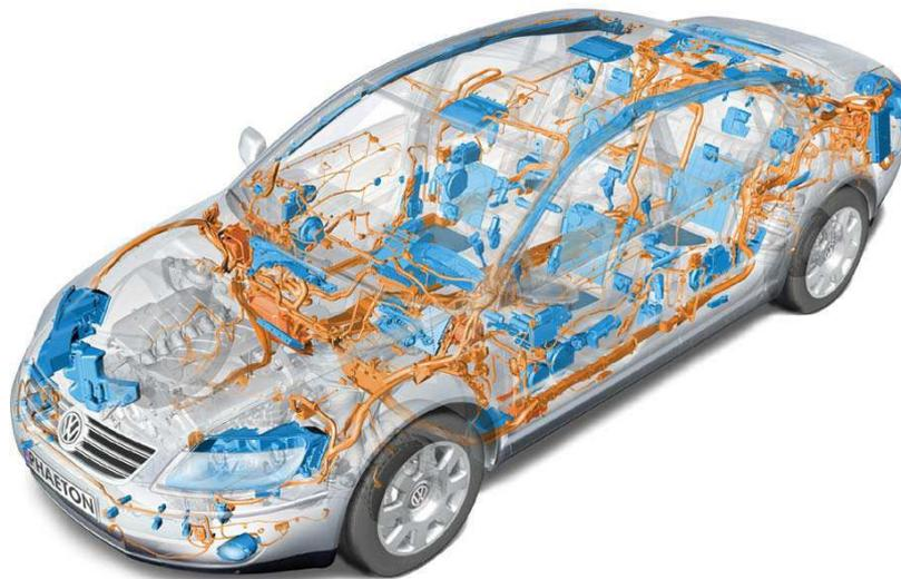
Figure 3.1: The electronic systems (blue) and communications channels (orange) in a Volkswagen Phaeton automobile (Image is from [149] and is courtesy of Volkswagen AG).
