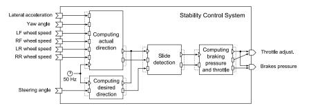
Figure 8.6: The SCS subsystem, modelled in ProSave.
