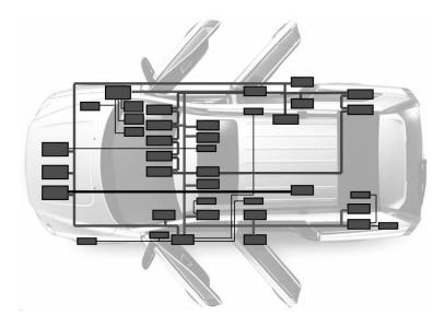
Figure 7.1: The electronic system architecture of Volvo XC90.
