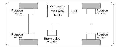
Figure 7.2: The ABS subsystem architecture.
