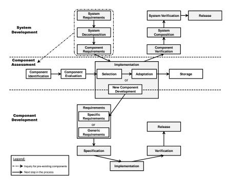
Figure 2.1: Component-based development process overview.
