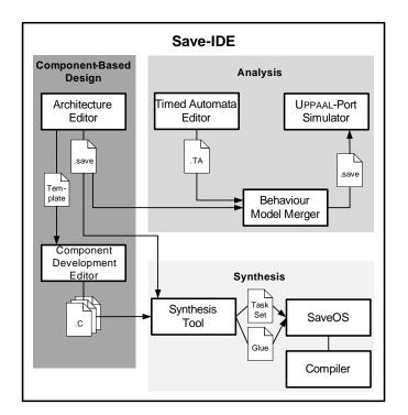
Figure 10.2: Overview of the Save-IDE tool-chain
