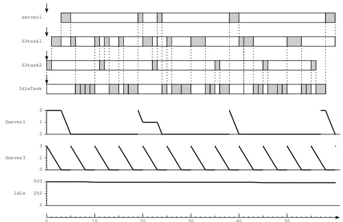
Fig. 16. Execution trace of HSF, running system1
