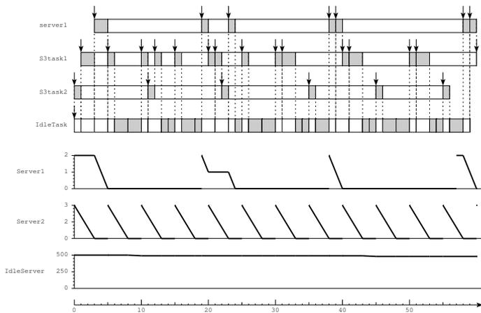
Fig. 18. Execution trace of TIMES scheduler (fragmented), running system 1
