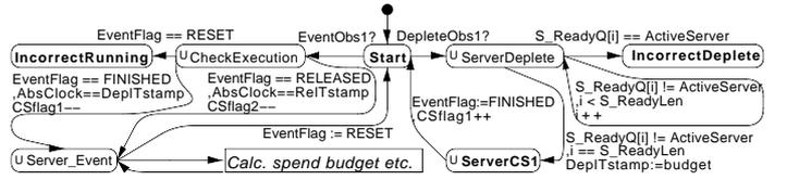
Fig. 13. *Observer1*: Server context-switch and depletion
