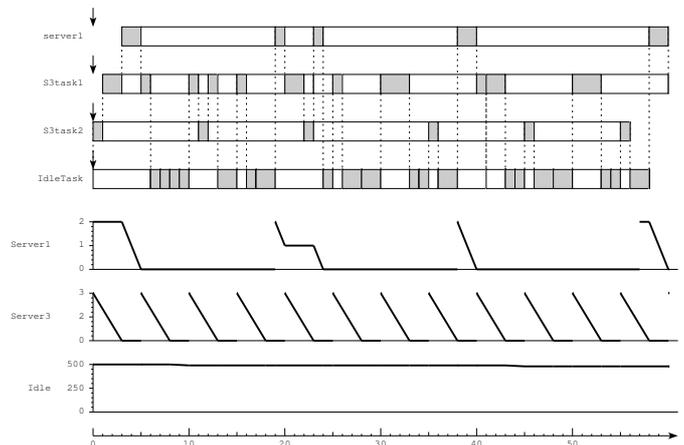
Fig. 17. Execution trace of TIMES scheduler (non-fragmented), running system1
