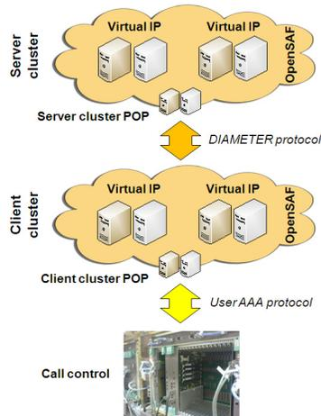
Figure 2. The deployment architecture of the demonstrator.
