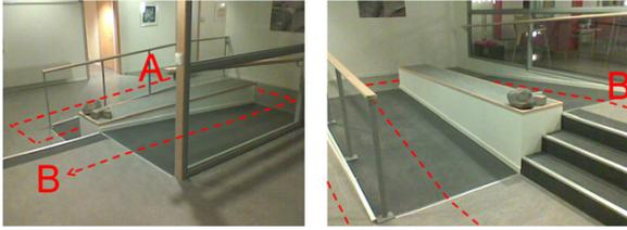
Fig. 8. S-shaped non planar path used to test the vSLAM algorithm. The path total length is 12 m, three 4m straight lines and three 1m diameter curves, covering 1 m difference in height.
