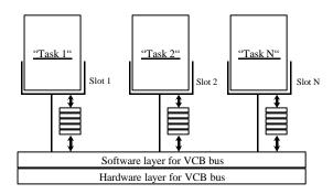
Figure 3 Logical architecture of a system with the VCB bus
