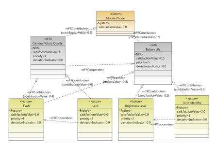
Figure 5.2: Example usage of NFR profile for a Mobile Phone (before calculations)
