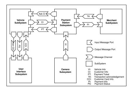
Figure 6.4: Component Model of the System using ProCom.
