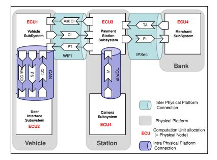
Figure 6.7: Deployment Model of the System depicting allocation to Physical Platforms.
