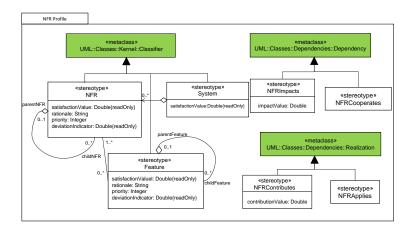
Figure 5.1: Profile for Trade-off analysis of NFRs
