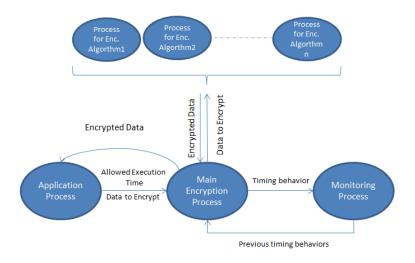
Figure 7.1: Adaptive design of encryption algorithms
