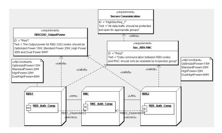
Figure 4.1: Security Requirement on RBS Nodes
