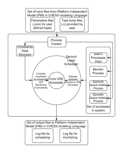
Figure 8.3: Components of The Design
