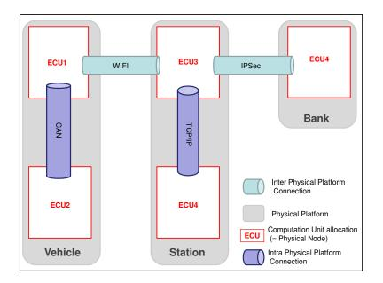
Figure 6.6: Physical Platform Model of the System.
