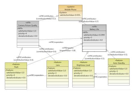
Figure 5.3: Analyzed model of the system
