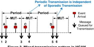
Figure 3. Mixed transmission pattern in HCAN
