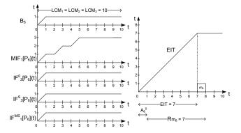
Figure 7. Demonstration for the calculation of response time of  $m_6$  from its reduced worst-case candidate 1
