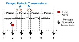
Figure 2. Mixed transmission pattern in AUTOSAR
