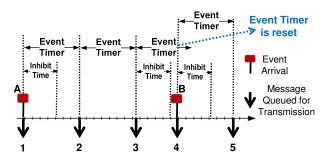
Figure 1. Mixed transmission pattern in CANopen
