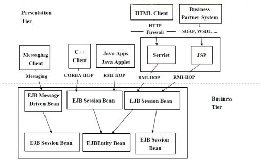
Figure 2: Client interaction with EJB component system
