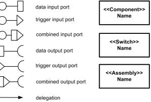
Figure 8: SaveCCM graphical notation
