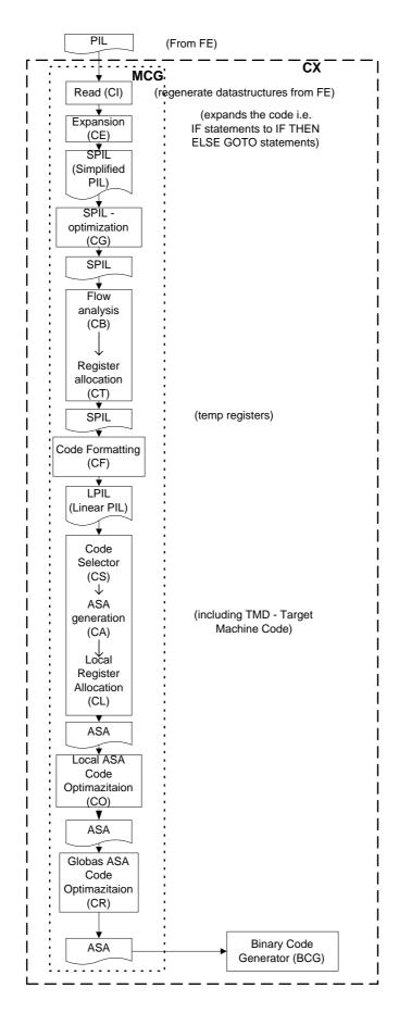
Figure 9.2: The structure of the back end. Input: PIL
