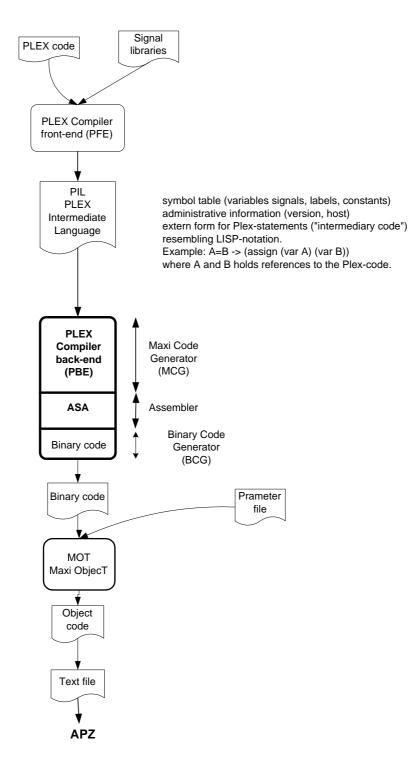
Figure 9.1: The structure of the compiler. Input: PLEX code (written by the programmer or compiled HL-PLEX code)
