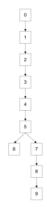
Figure 11.6: The corresponding depth-first spanning tree.
