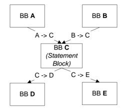
Figure 9.3: A DO Statement block with multiple entries (from other Basic Blocks (BB)) and multiple exits (to other BB). The notation  $A \rightarrow C$  indicates that the edge is a path from A to C.
