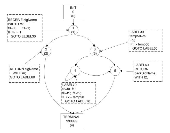
Figure A.1: The control flow-graph before loop elimination for program: fib.program.
