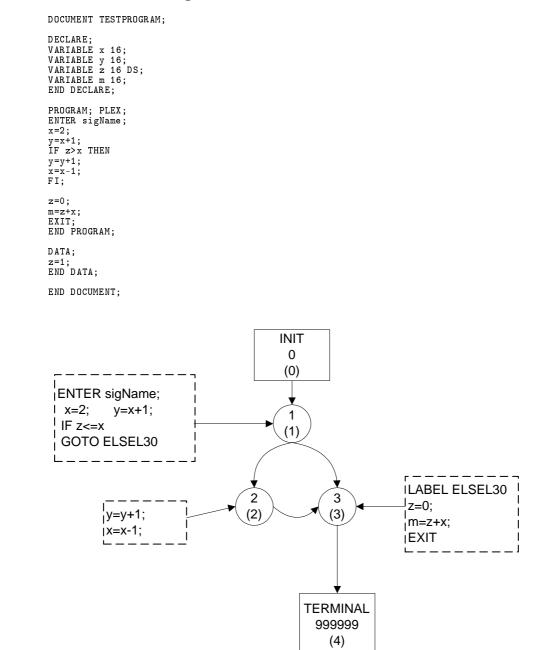
Figure A.3: The control flow-graph for program: test1.program.
