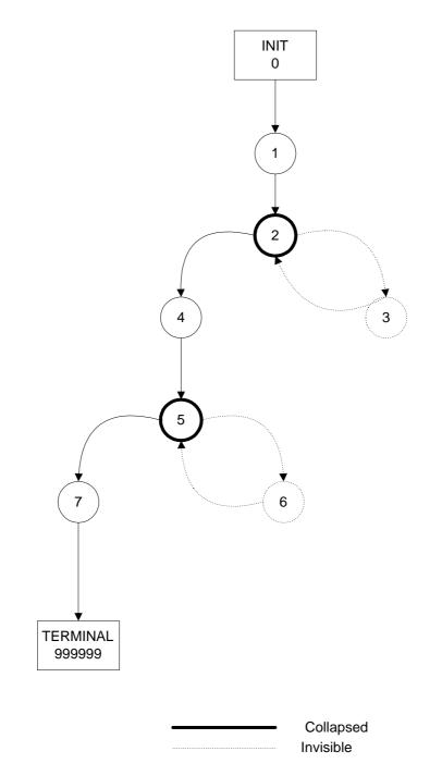
Figure 12.2: The control flow-graph after loop elimination for program: clear\_assign.program.
