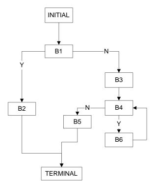
Figure 5.2: The flow-graph for fig 5.1
