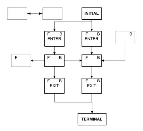
Figure 9.4: The basic blocks are traversed and marked if visited. F - visited on forward traversal, B - visited on backward traversal. Dashed basic blocks constitute dead basic blocks.
