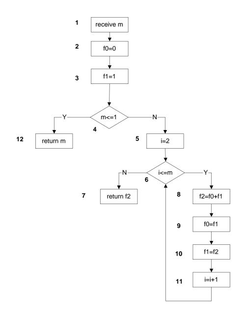
Figure 5.1: The graph for the Fibonacci code.
