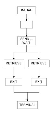
Figure 9.5: The control flow-graph before the handling of destructive statements.
