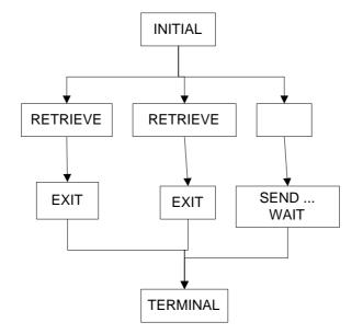
Figure 9.6: The control graph in 9.5 after the destructive statements have been handled.
