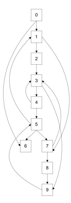
Figure 11.7: The depth-first spanning tree with the remaining edges added.
