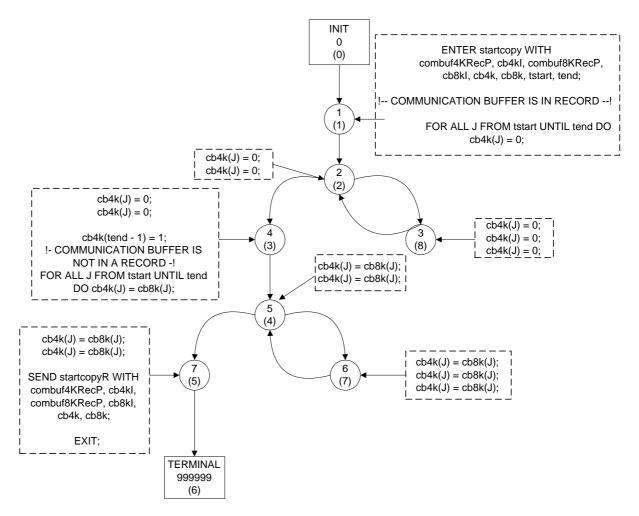
Figure 12.1: The control flow-graph before loop elimination for program: clear assign.program.
