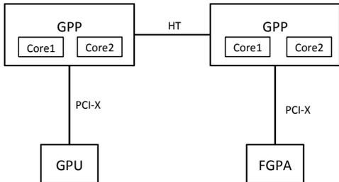
Figure 1: Example of heterogeneous system
