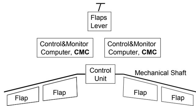
Figure 3. Overview of the High Lift System
