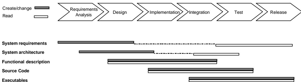
**Figure 2. SW design process and information usage**
