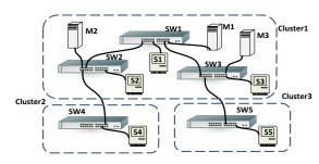
Fig. 6. A Network with Five Switches
