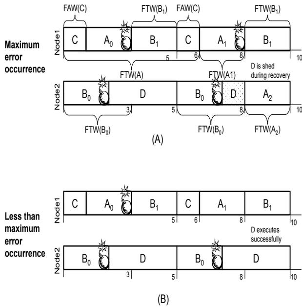
Fig. 3. (A). Allocation and execution under worst case error scenario (B). Allocation and execution under average case error scenario
