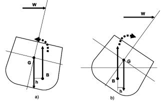
Figure 1. Stable and unstable attitudes of a ship
