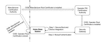
Figure 2. High Level View on Home Base Station Authentication
