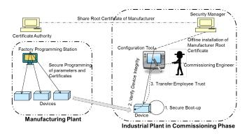
Figure 4. Overview of Proposed Device Authenticity Verification
