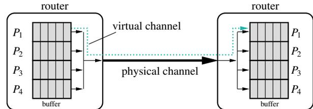
Figure 1: Virtual channels on the NoC router.
