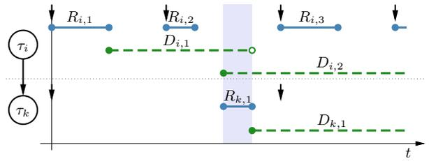
Fig. 6: Read and data interval of  $\tau_i$  and  $\tau_k$ , if they are dependent through a precedence constraint  $\tau_i \xrightarrow{(2,1)} \tau_k$ .
