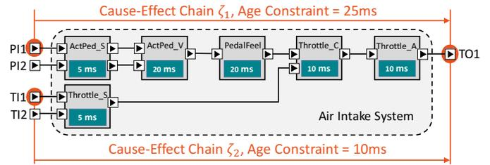
Fig. 10: Component view of the AIS of an Engine Management System.
