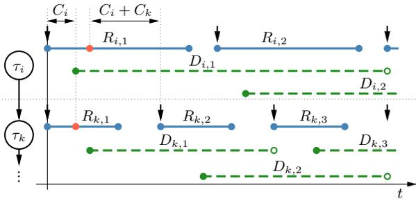
Fig. 5: Required modifications to the read interval of job  $\tau_{i,1}$  and job  $\tau_{k,i}$ , if they are dependent through a precedence constraint  $\tau_i \xrightarrow{(1,1)} \tau_k$ .
