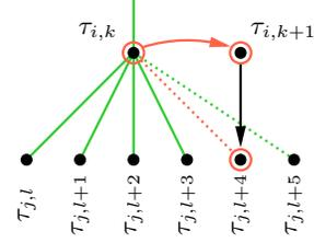
Fig. 8: Adding a job-level dependency to prune invalid data paths.
