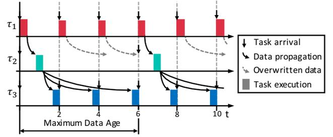
Fig. 2: Data propagation paths and maximum data age in a real-time system.
