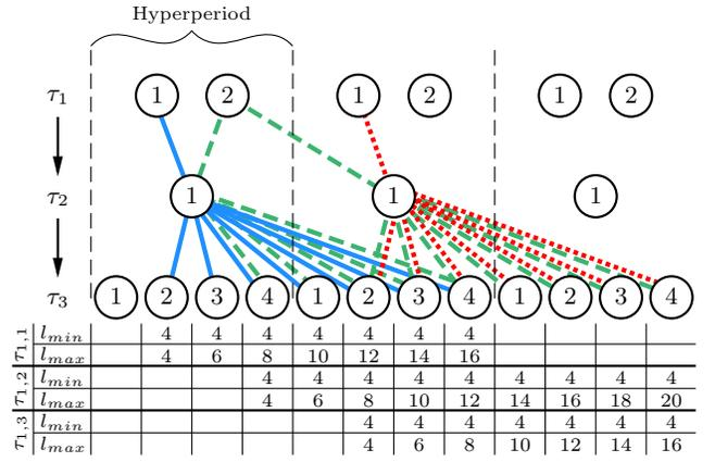
Fig. 7: Cause-effect chain  $C$  and the data propagation trees for the first three instances of  $\tau_1$ . Minimum and maximum latencies  $l_{min}$  and  $l_{max}$  for each data propagation tree is shown in the table.
