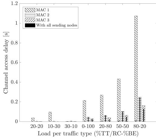
Fig. 8. Average channel access delay for the different MAC protocols under different loads and distributions of load. For MAC 2 and MAC 3, only the best configurations are shown (MAC 2B and MAC 3B). Thin black bars represent the case when traffic comes from all nodes.
