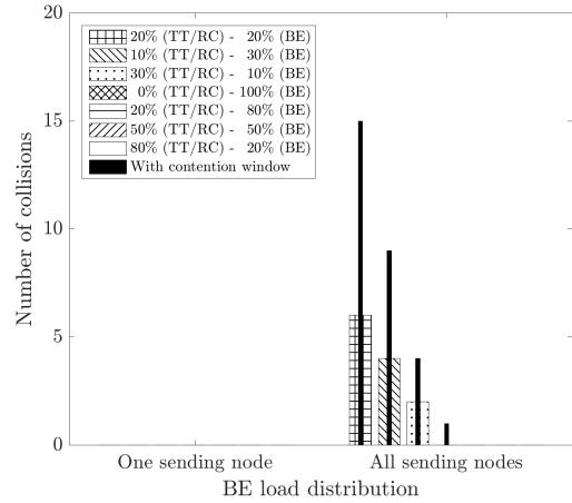
Fig. 5. Number of collisions for MAC Protocol 2A for different loads and distributions of load. Thin black bars are for MAC 2B.
