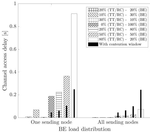
Fig. 4. Average channel access delay for MAC Protocol 2A for different loads and distributions of load. Thin black bars are for MAC 2B.
