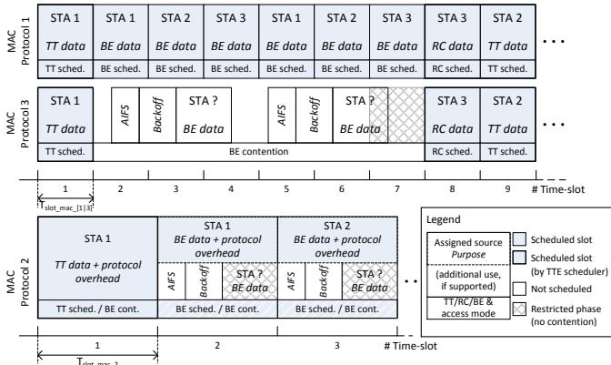
Fig. 2. Traffic scenario example for the proposed wireless MAC protocols.
