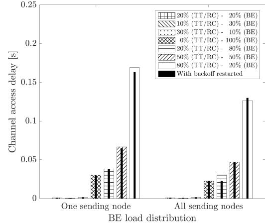
Fig. 6. Average channel access delay for MAC Protocol 3A for different loads and distributions of load. Thin black bars are for MAC 3B.
