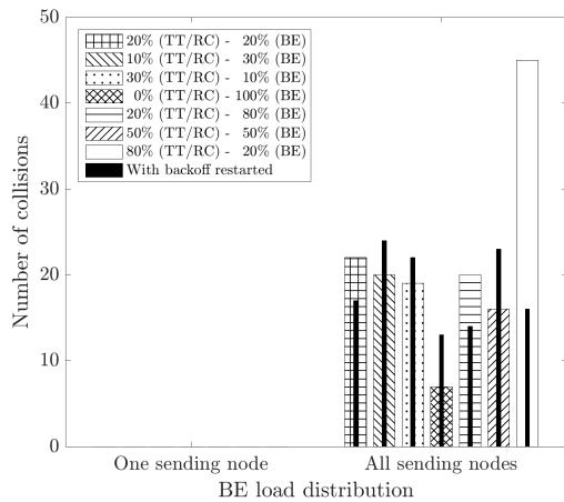
Fig. 7. Number of collisions for MAC Protocol 3A for different loads and distributions of load. Thin black bars are for MAC 3B.
