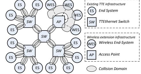
Fig. 1. Example of the proposed wired-wireless scenario, with switches (SW) and access points (AP) connecting the end-systems (ES, WES) forming recursive star topologies (snowflake topology). Note that every wired connection forms two collision domains, while the wireless systems constitute a single collision domain.
