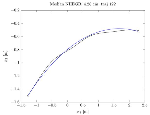
**Fig. 11** A comparison between the path, corresponding to the median distance error, generated with cost function (5) (black line) and the corresponding experimental path (blue line). The ‘o’ and ‘x’ indicate the initial and final position, respectively (Color figure online)
