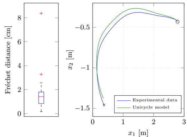
**Fig. 5** A comparison between the paths generated using the unicycle model and the experimental paths: on the *left side* the box-plot of the validation error, on the *right side* the simulated (*green line*) and experimental (*blue line*) paths corresponding to the worst outlier. The ‘o’ and ‘x’ indicate the initial and final position, respectively (Color figure online)
