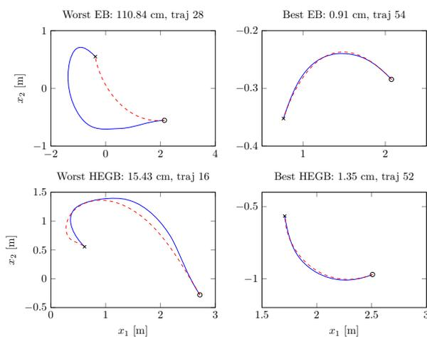
**Fig. 7** The best and the worst path generated with the EB and with the HEGB approaches. The solid lines represent the experimental paths, the dashed lines are the optimal EB and HEGB solutions, and the ‘o’ and ‘x’ indicate the initial and final position, respectively
