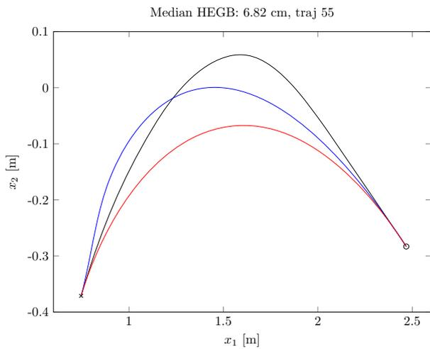
**Fig. 9** A comparison among the paths, corresponding to the median distance error, generated with the EB (red line) and the HEGB (black line) approach and the corresponding experimental path (blue line). The ‘o’ and ‘x’ indicate the initial and final position, respectively (Color figure online)
