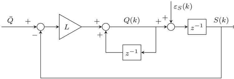
Fig. 4 Block diagram of the controller of SAS servers
