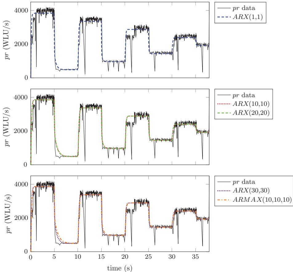
Figure 4. Identification results for the vips software application with different model structures. The data used for the identification are denoted with a solid line, the simulation results of the ARMAX (10, 10, 10) with a dashed-dotted line, the ARX (30, 30) with a densely dotted line, the ARX (20, 20) with a densely dashed line, the ARX (10, 10) with a densely dotted line, and the ARX (1, 1) with a dashed line.
