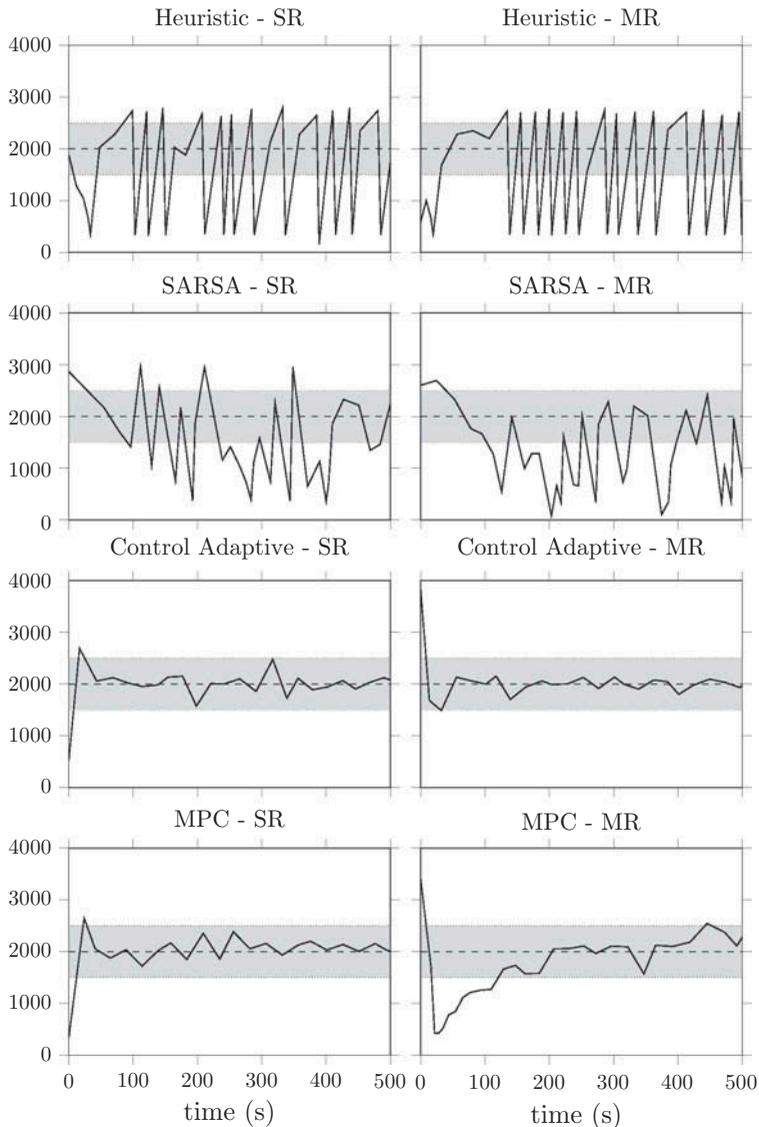
Figure 6. Experimental results with different model-based/non-model-based techniques. Note: SARSA, State-Action-Reward-State-Action; MPC, Model Predictive Control.
