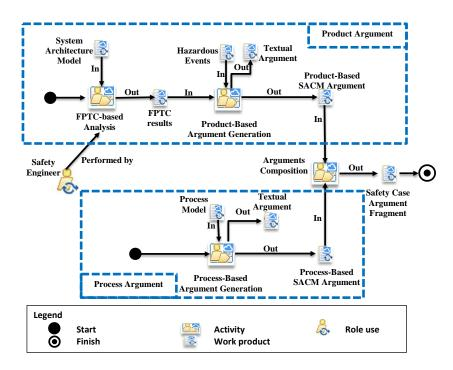
Fig. 8 Safety process modelled using EXE-SPEM. Adapted from [4]
