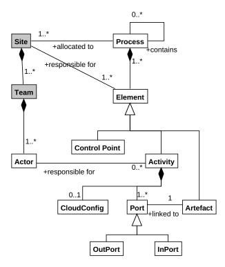
Fig. 5 The software process model XML schema
