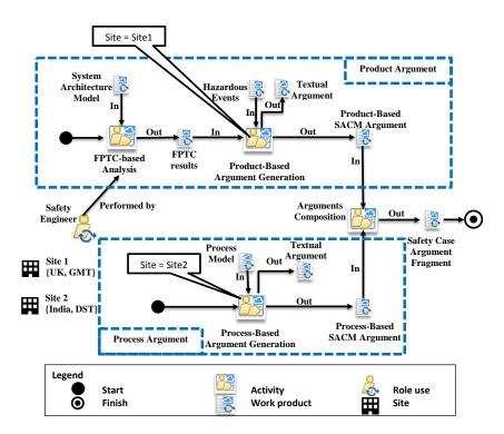
Fig. 9 Safety process modelled using the extended EXE-SPEM
