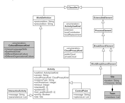
Fig. 4 The extended meta-model of EXE-SPEM
