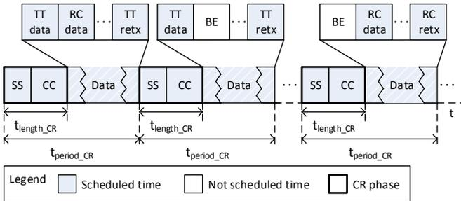
Fig. 2. CR phases allocation in the MAC. An example for the data allocation is also provided.
