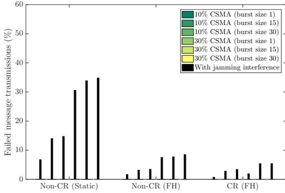
Fig. 5. Percentage of failed messages for non-CR and CR-based MAC following the Consecutive time diversity scheme.
