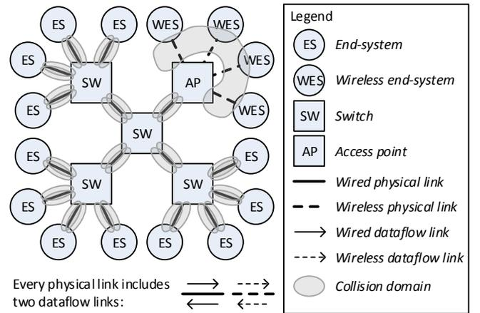
Fig. 1. Example of hybrid wired-wireless multi-hop network with snowflake topology.
