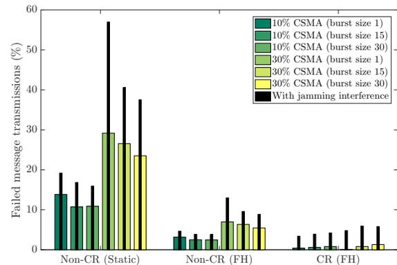
Fig. 4. Percentage of failed messages for non-CR and CR-based MAC without time diversity.
