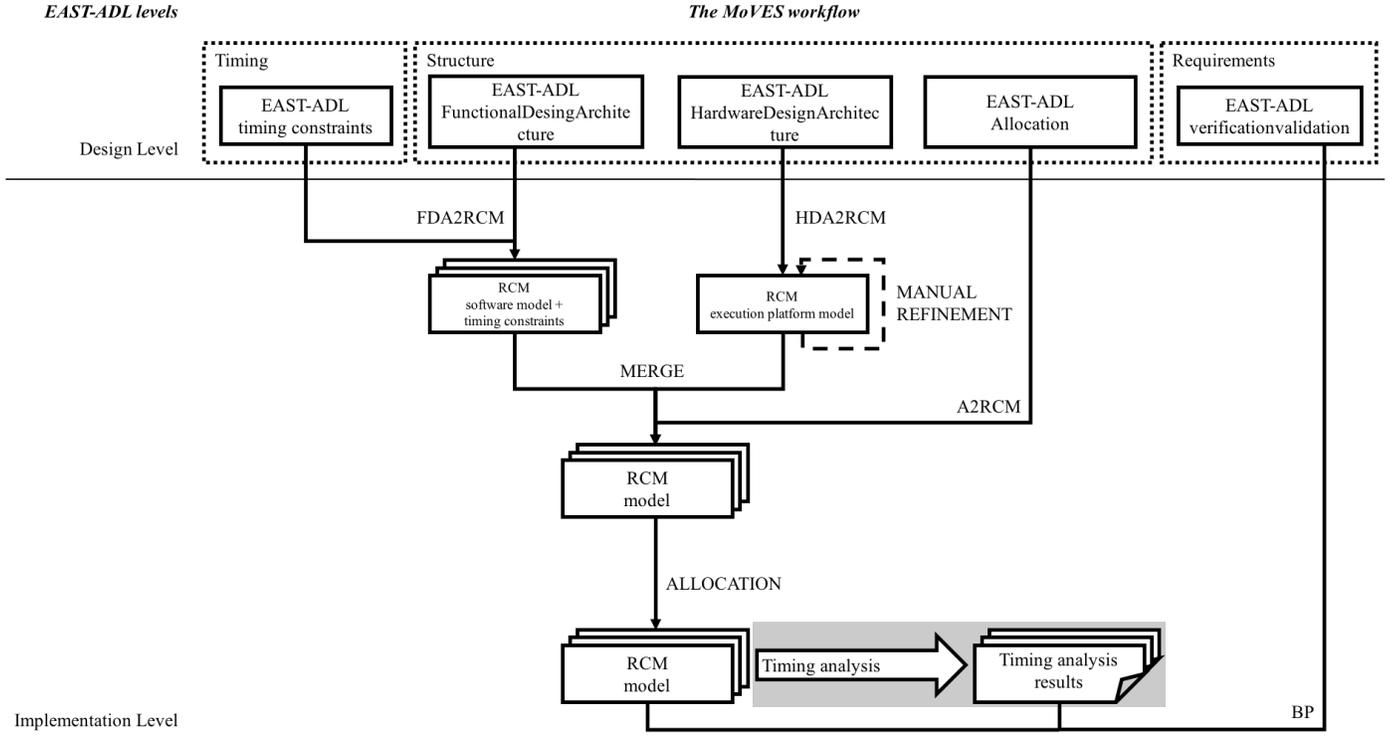
Fig. 7: The MoVES and its composing tasks
