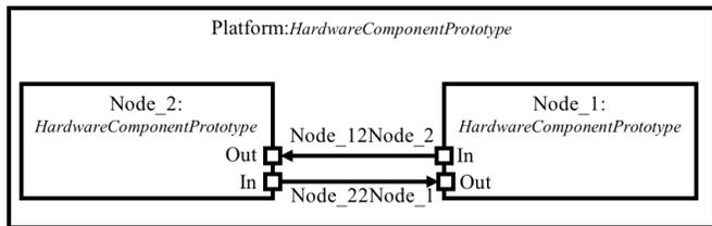
Fig. 16: EAST-ADL HardwareDesignArchitecture of the ACC system
