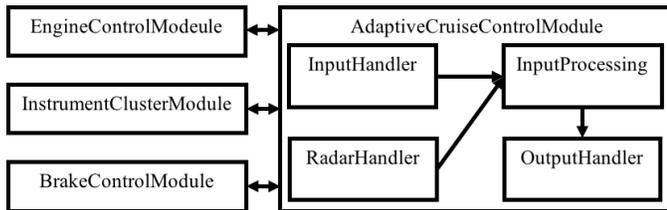
Fig. 13: Block diagram of the ACC system.
