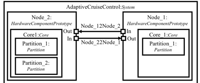
Fig. 17: RCM execution platform model of the ACC system
