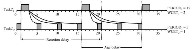
Fig. 5: Example showing end-to-end delays
