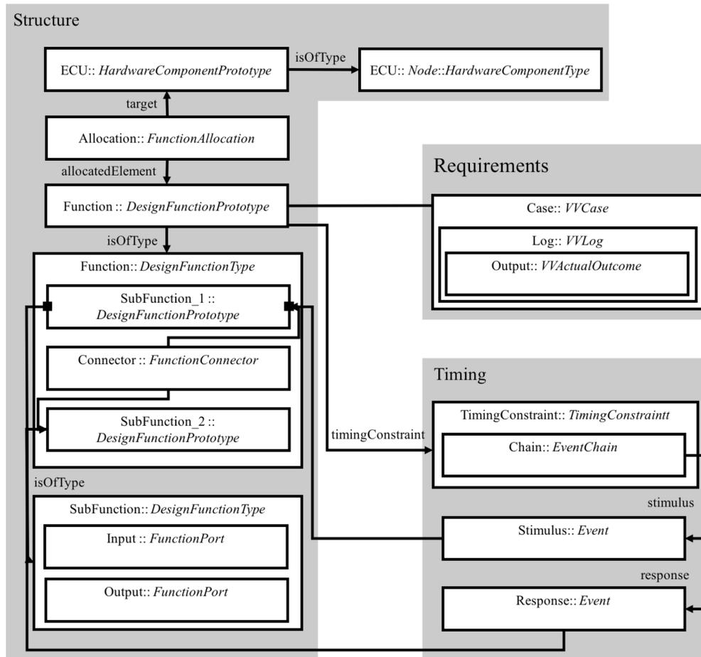
Fig. 1: Simplified EAST model containing concepts from the EAST-ADL structure, timing and requirements packages
