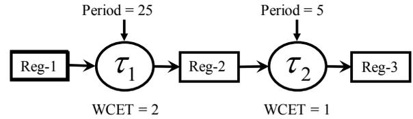
Fig. 4: A task chain with independent activations of tasks
