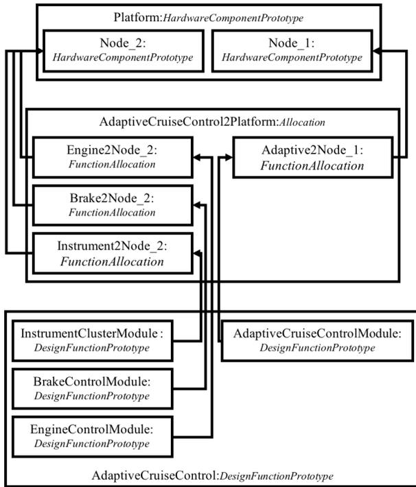
Fig. 18: EAST-ADL Allocation of the ACC system
