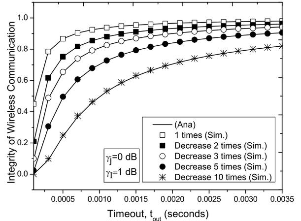
Fig. 4. Transmission Probability vs. Decreasing Channel Gains over Time
