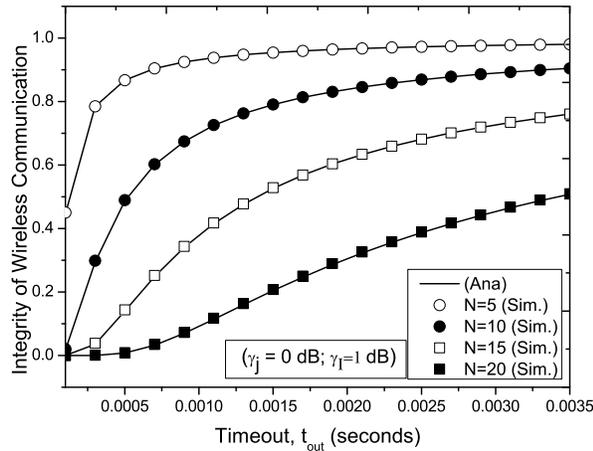
Fig. 5. Number of vehicles vs. system performance
