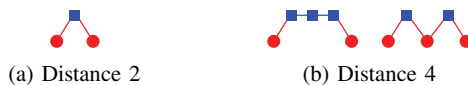
Figure 4: Examples of test case to test case distances. Red circles are test cases, and blue squares are requirements.
