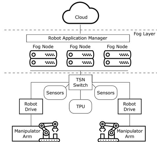
**Figure 2: Proposed fog based architecture for Industrial Robotic System.**
