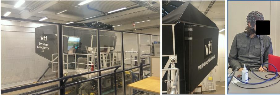
Figure 3.1: VTI simulator III and EEG electrodes setup on a participant.
