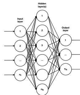
Fig. 2. An illustration of Multi-layered Perceptron.
