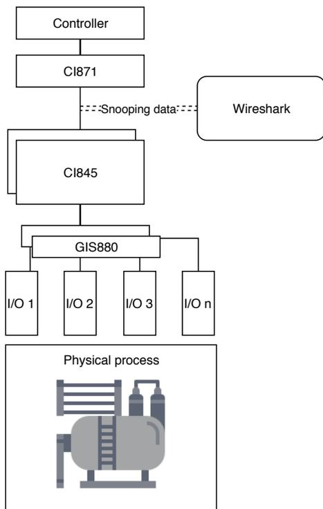
Fig. 1. System setup of the ABB Select I/O™.
