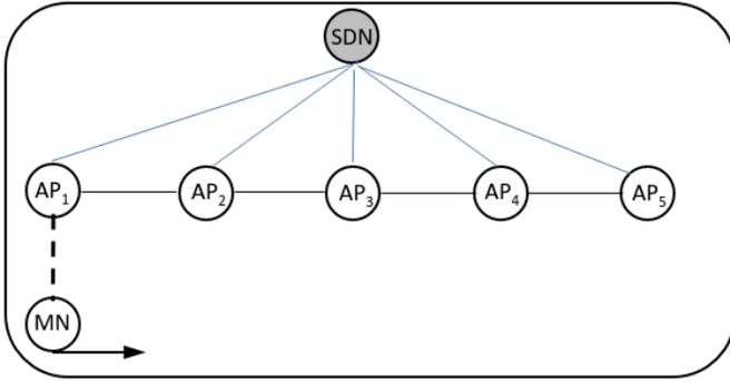
Fig. 3. A Fog computing IoT architecture with an SDN controller, a set of APs and a mobile node.
