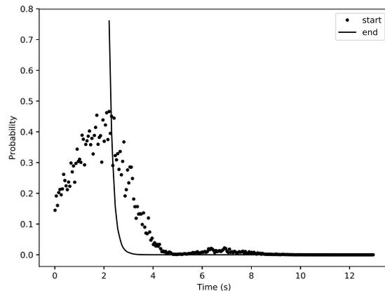
Fig. 6. Probability of starting handoff as indicated by dots, gets to its maximum after 2.2 seconds. Assuming that seamless handoff starts at that specific time slot, the conditional probability of ending the handoff as shown by the line, is high at exactly the same time instance.
