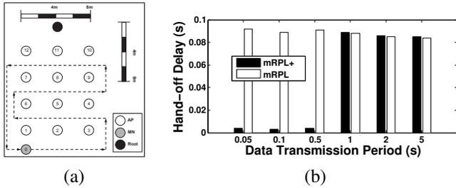
Fig. 1. (a) nodes' deployment, and (b) handoff delay of mRPL and mRPL+ with different data transmission periods [7].
