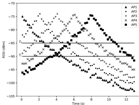
Fig. 5. The RSSI measured at the APs when the MN moves with a constant speed of 1m/s and the APs are statically placed at specified locations, as in Figure 3.
