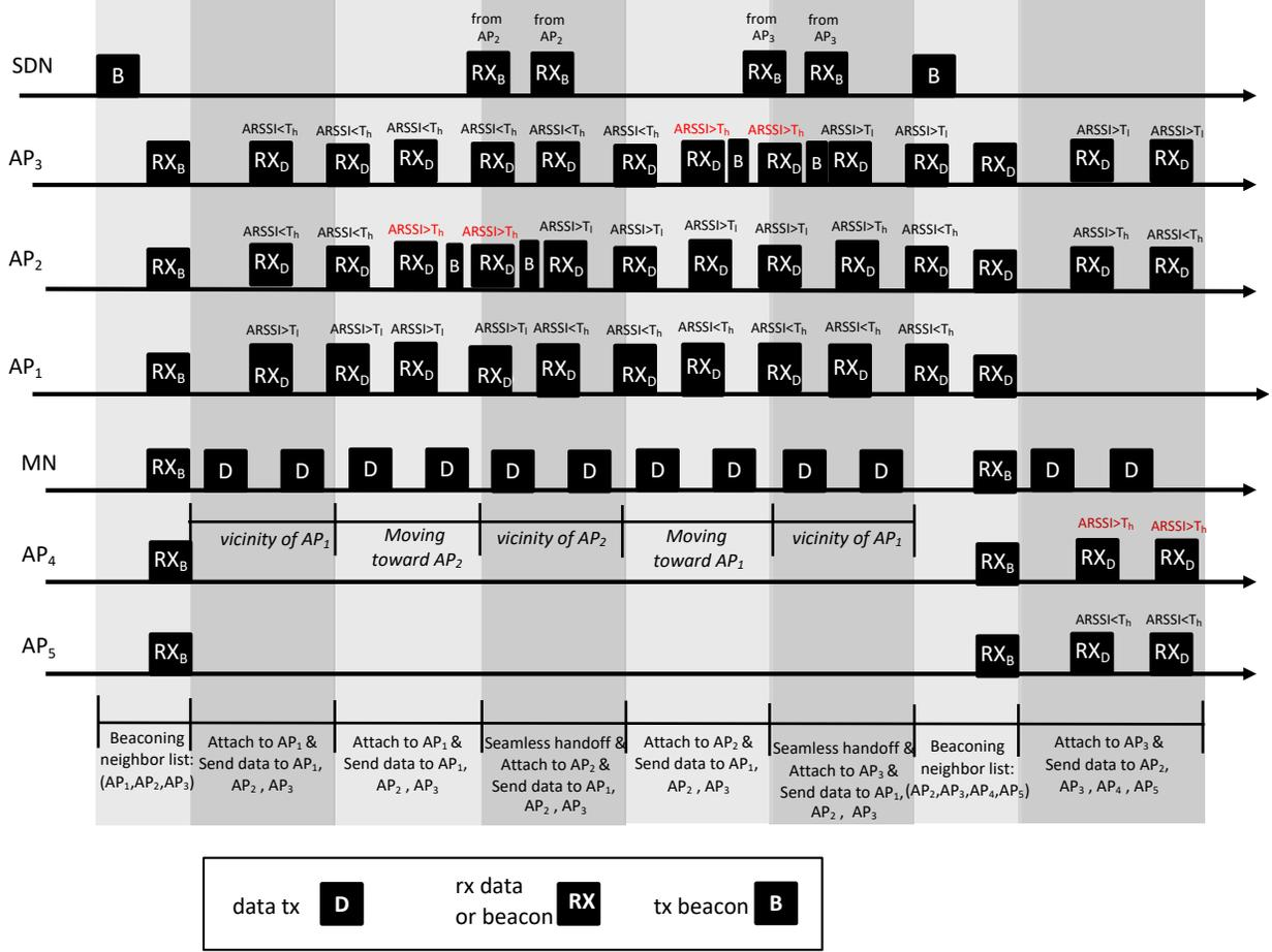
Fig. 4. As the MN moves across the horizontal path, the corresponding ARSSI changes over time and there is no need for any beaconing in the seamless handoff but if the parent that is the MN is going to attach to, does not exist in the MN's parent list a beacon from the SDN is required.
