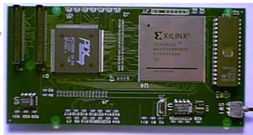
Block diagram of SARA-System and Picture of a RTU-PMC board
