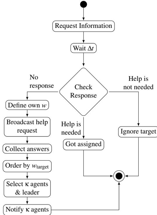
Fig. 2: Activity diagram of the agent's behaviour when a new target is spotted [12].
