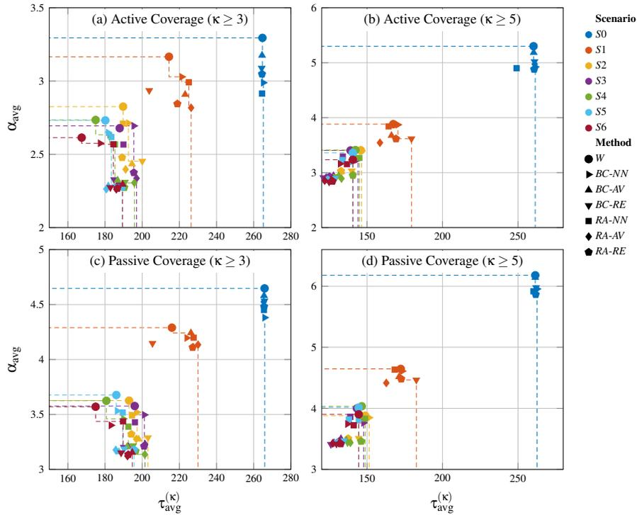
Fig. 6: Average number of agents covering targets vs average coverage time of all targets of the entire duration of the simulation for  $\kappa \geq 3$  and for  $\kappa \geq 5$ . On the top we show active coverage where we only consider the agents actively following a target while the bottom includes passive coverage — agents having multiple targets in their visibility range while following another target [12].
