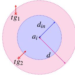
Fig. 3: Agent  $a_i$  with visibility range  $d$ , indicated with the red circle, and internal range  $d_{in}$ , indicated with the blue circle. The targets  $tg_1$  and  $tg_2$  are indicated with crosses, and they are moving towards and away from the agent, respectively [12].
