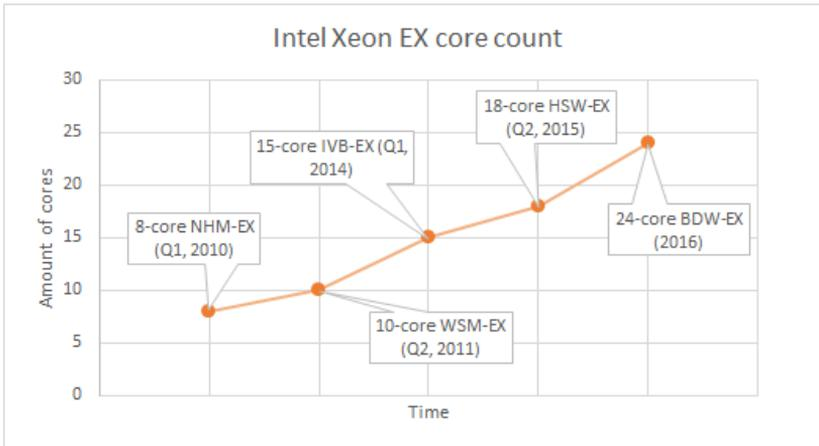
**Figure 1.2:** Intel® Xeon core development between 2010 and 2016
