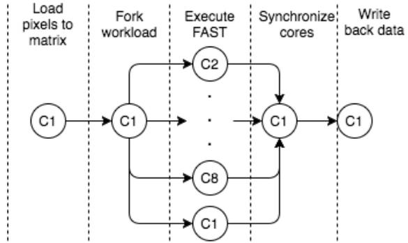
**Figure 7.3:** FAST 8 core execution model
