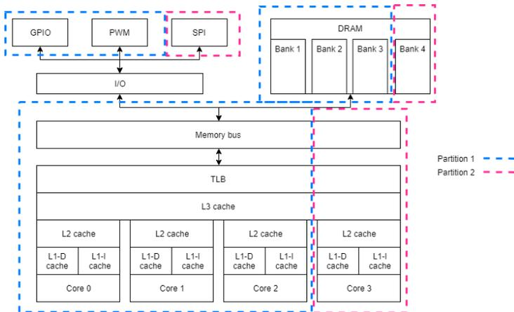
**Figure 2.12:** Example of a completely partitioned system
