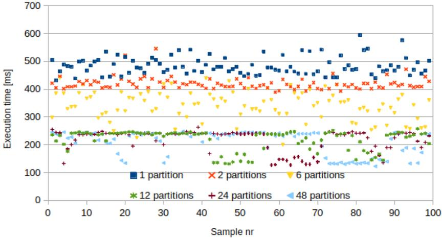
**Figure 5.4:** Matrix multiplication using different cache partition sizes
