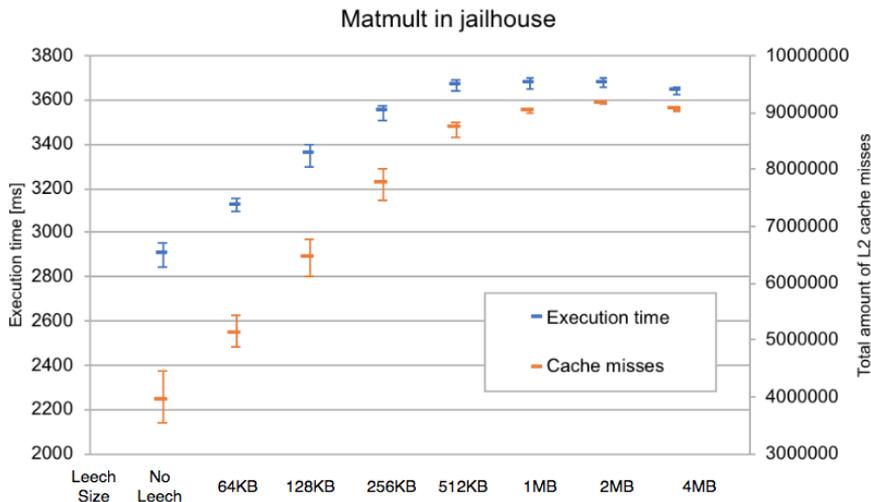
**Figure 9.4:** Jailhouse L<sub>2</sub>-cache isolation test
