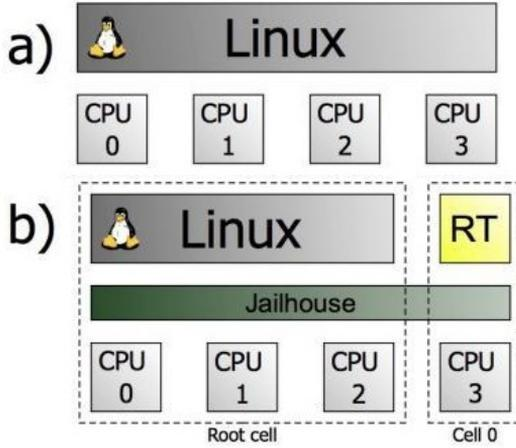
**Figure 9.1:** a) Usual Linux deployment. b) Linux with Jailhouse configuration [15]
