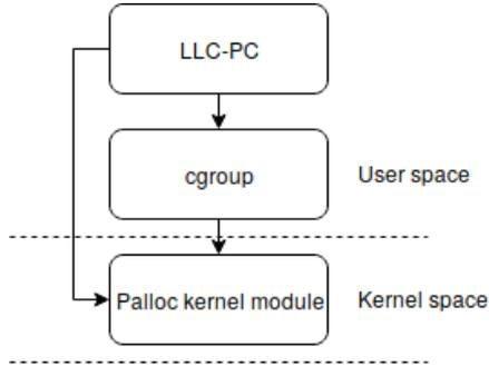
**Figure 10.5:** System connections
