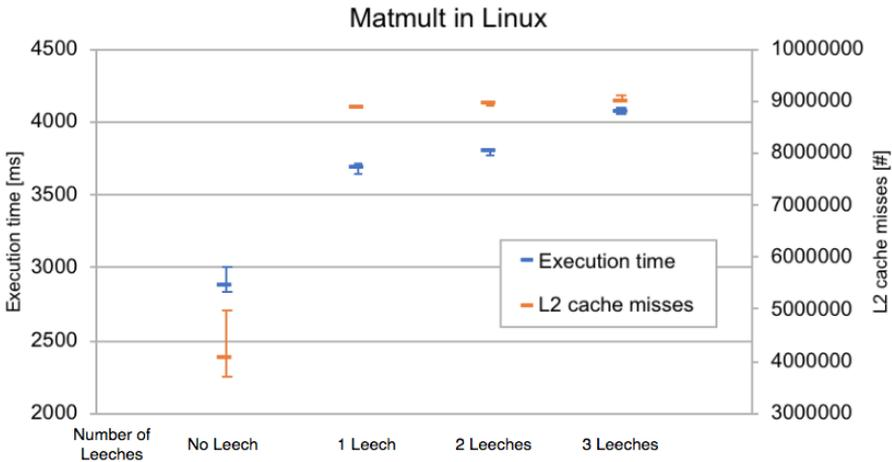
**Figure 9.5:** Linux memory bus isolation test
