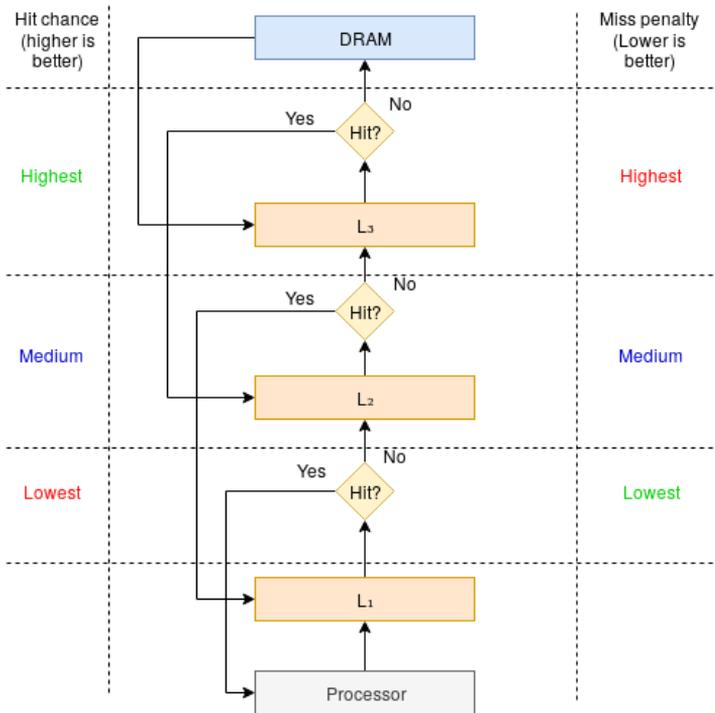
**Figure 2.7:** Three-level cache lookup procedure
