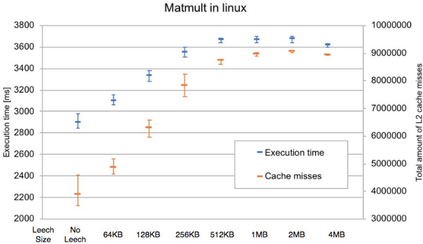
Figure 9.3: Linux L<sub>2</sub>-cache isolation test
