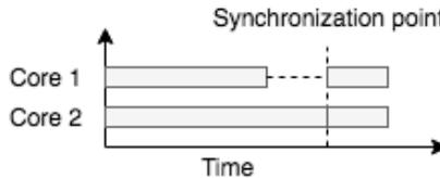
**Figure 7.4:** Core idle issue due to synchronization
