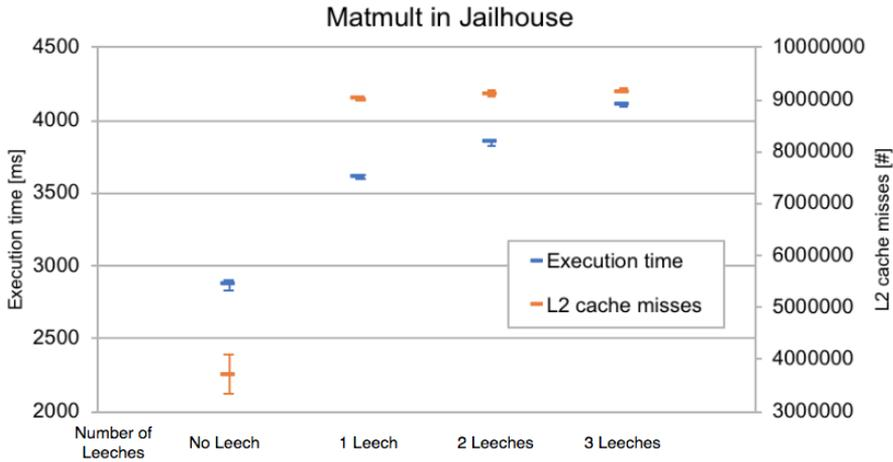
**Figure 9.6:** Jailhouse memory bus isolation test
