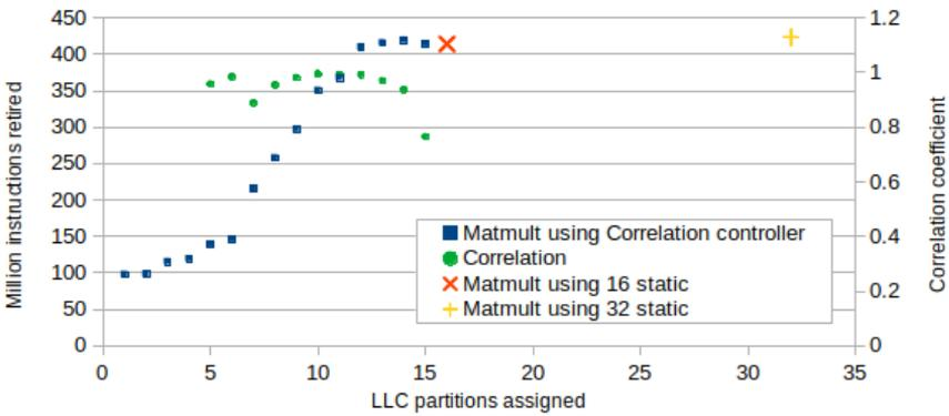
**Figure 10.9:** Comparison of 756x756 matrix multiplication executions
