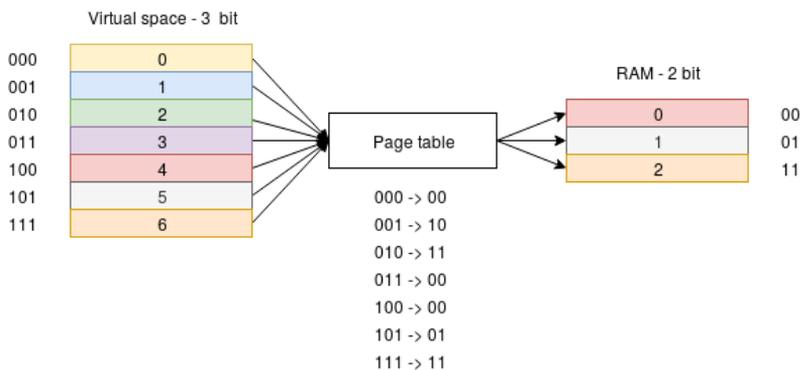
**Figure 2.3:** Illustration on page table mapping
