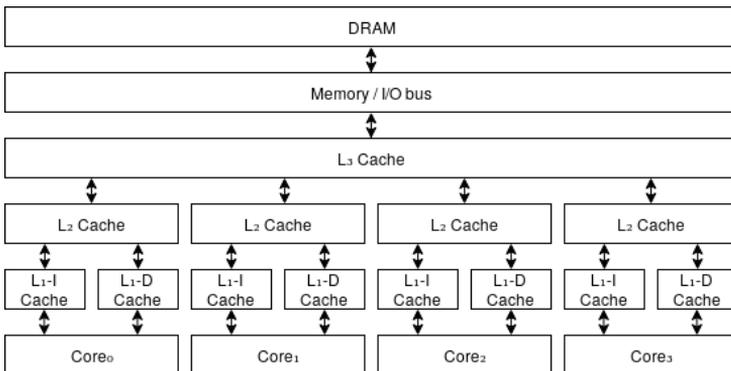
**Figure 1.1:** Example of a typical Intel<sup>®</sup> 4-core system
