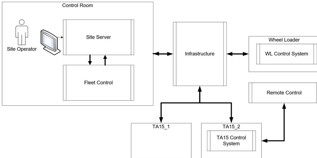
Fig. 2. Interaction of control systems in a system-of-systems
