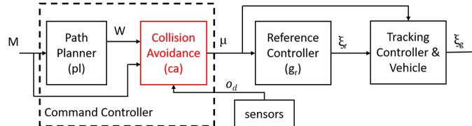
**Fig. 3.** The architecture of the controller of autonomous vehicles
