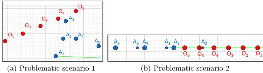
**Fig. 11.** Problematic scenarios discovered by counter-examples. AV’s discretized trajectory is blue dots. The dynamic obstacle’s discretized trajectory is red dots. AV’s reference path is the green line. For differentiation, positions that are too close but belong to different time points are represented by small and large dots in scenario 2.  $A_n$  and  $O_m$  indicate the AV and obstacle, respectively,  $n$  and  $m$  are time points.
