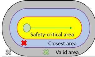
**Fig. 10.** The green arrow is the reference path. The green circle is the AV. The crosses are the dynamic obstacles, where red and grey ones are invalid positions, and the green cross is valid.
