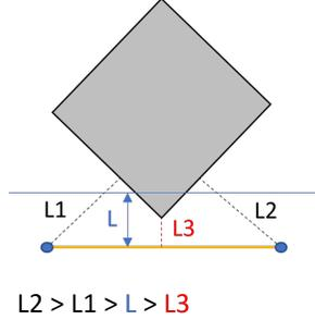
**Fig. 12.** A special case where the distances from the two ends of a line segment do not represent the distance from the static obstacle to the line segment.
