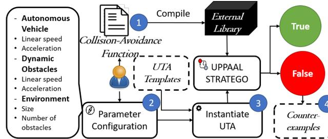
Fig. 7. The workflow of the verification approach
