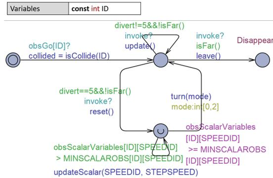
Fig. 14. The UTA template of dynamic obstacle movement
