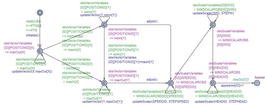
Fig. 13. The UTA template of dynamic obstacle initialization
