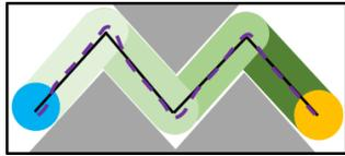
**Fig. 2.** The reference trajectory of the AV’s position is depicted as solid black lines, and the actual trajectory is depicted as violet dotted lines. The boundaries of tracking errors are green. Static obstacles are grey [10].
