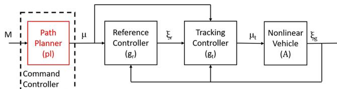
**Fig. 1.** A controller of autonomous vehicles without a collision-avoidance module
