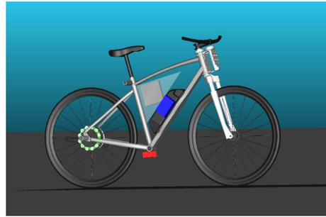
Fig. 4. The instrumented bicycle designed in SolidWorks and imported to Adams is used as the plant in the co-simulation between Adams and Matlab.
