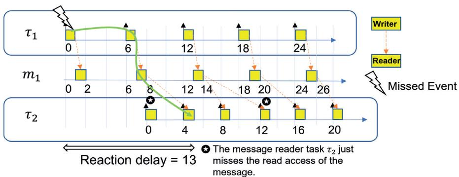
**Figure 2.9:** A possible execution trace for the distributed embedded system example shown in Figure 2.6 when source and destination are not synchronized (reaction delay).
