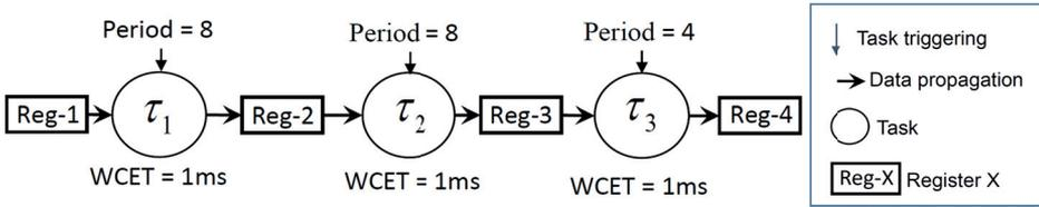
**Figure 2.4:** An example of a task chain that uses register-based communication.
