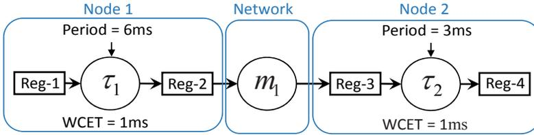
Figure 2.6: A multi-rate chain in a distributed embedded system.
