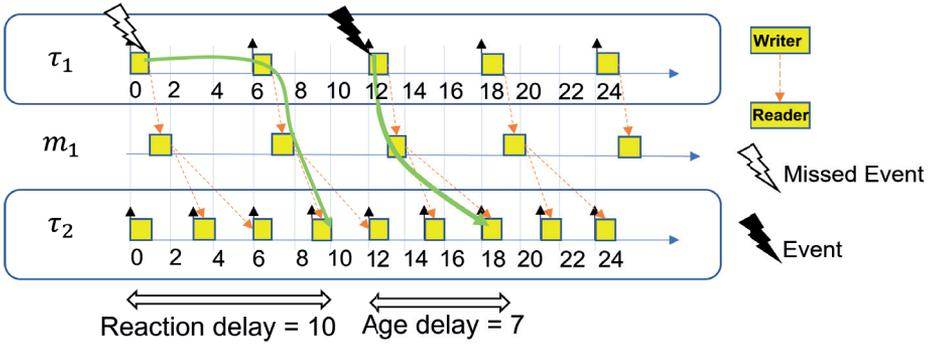
**Figure 2.7:** A possible execution trace for the distributed embedded system example shown in Figure 2.6 when source and destination nodes are synchronized.
