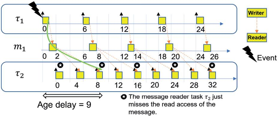
**Figure 2.8:** A possible execution trace for the distributed embedded system example shown in Figure 2.6 when source and destination nodes are not synchronized (age delay).
