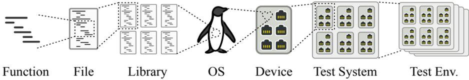
**Figure 1.4:** Perspectives of testing: from low level (source code functions) to high level (system).
