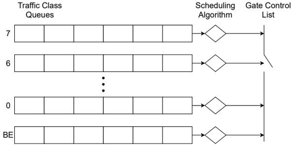
Fig. 1: A TSN bridge model with the traffic class queues, transmission scheduling algorithm and gate control list.
