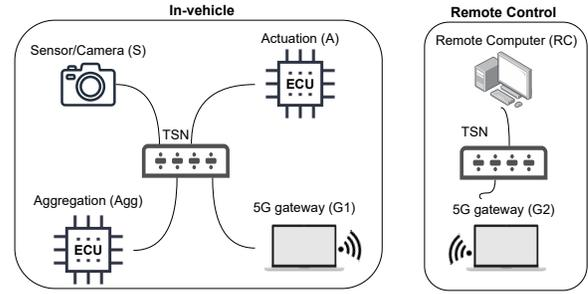
Fig. 8: Automotive industrial use case utilizing TSN & 5G.
