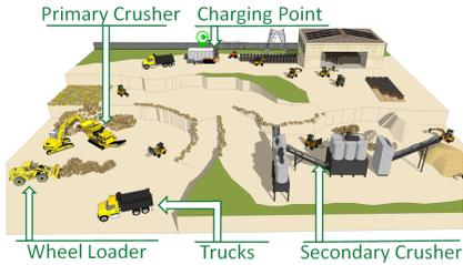
Figure 3: An autonomous quarry
