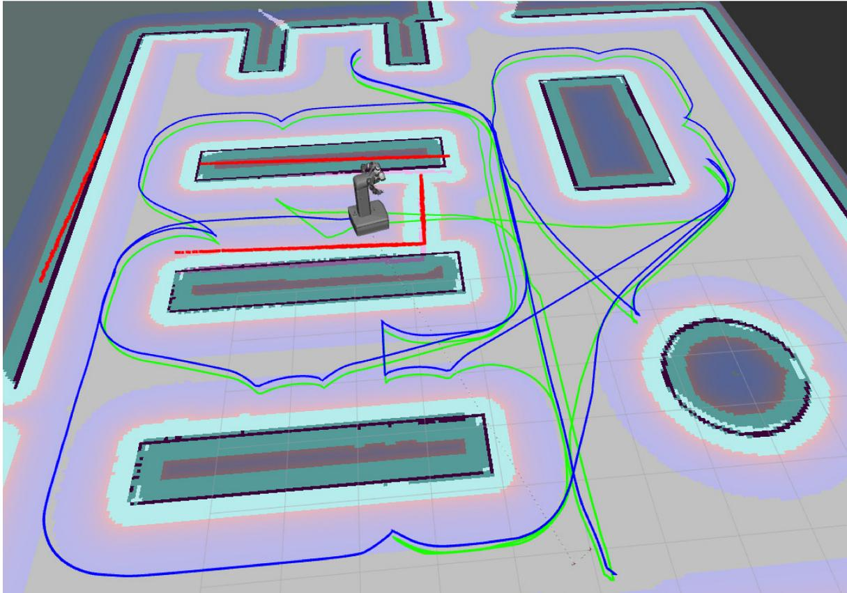
**Figure 3.** Warehouse layout. The light green path, starting and ending at the bottom right, is the initial route for Scenario B. The robot has stopped in front of an obstacle that is blocking the initially planned movement. The red lines along the shelves, the wall and the obstacle indicate the objects perceived by the robot’s laser scanner. A replanned route in blue, starting at the robot’s location, has changed the order of the remaining tasks.
