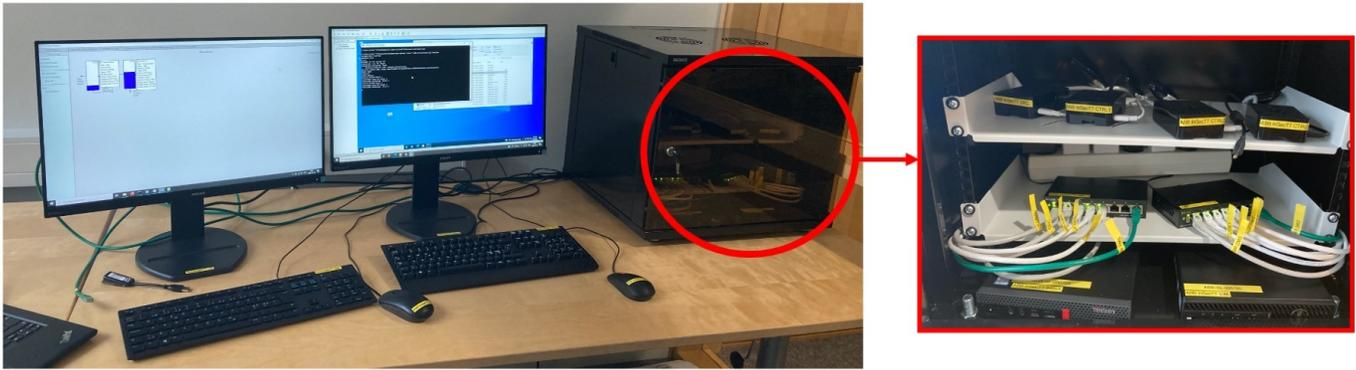
Fig. 5: Lab environment setup which includes hardware of the ice-cream factory example, with two modules simulated.
