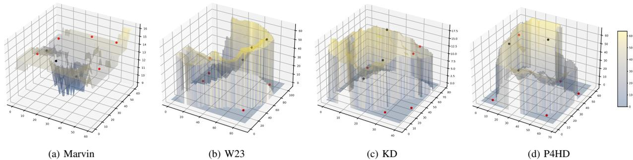
Fig. 6: Snapshots of the initial states of the mines and the deployment of fixed BSs in (a) Marvin (b) W23 (c) KD and (d) P4HD mines. The red and blue dots represent the fixed BSs and CoWs, respectively. For Zuck and SM2 timelines of the topography are provided in Fig. 7 and 8. The measurement unit for all 3 axes is the number of blocks. The colors also represent the height of the terrains.
