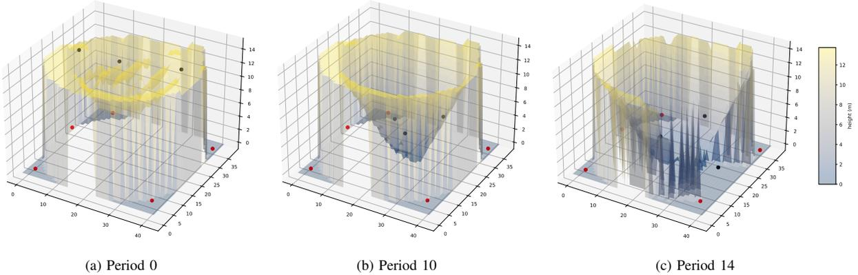
Fig. 8: Evolution of the Zuck mine and deployment of 5 fixed BSs (red dots) and 3 CoWs (black dots). Zuck presents special constraints for the radio network deployment since the highest parts of the terrain act as obstacles and only get extracted in the final phases.
