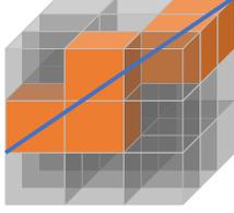
Fig. 3: 3D Bresenham algorithm projects the line between the BS and the target on a 3D mesh.
