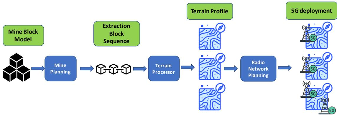
Fig. 2: The flow of information in different modules of the optimization framework. The CPIT module takes the initial block model of the mine and generates a sequence of blocks that need to be extracted. This extraction sequence is then used to calculate the terrain profile based on which the radio planning is performed.
