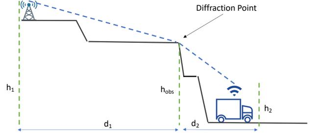
Fig. 4: Diffraction point and the relative height of the transmitter and receiver.
