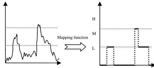
Figure 1: Mapping various kind of traffic specification to few QoS levels
